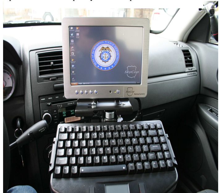
SkyCop Adjustable Mounting System for Touch Screen Monitor & Backlit Keyboard or Laptop Computer
