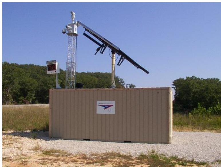
On-Board Radar Detection, License Plate Recognition, and Thermal Imaging Camera Fort Leonard Wood Missouri
